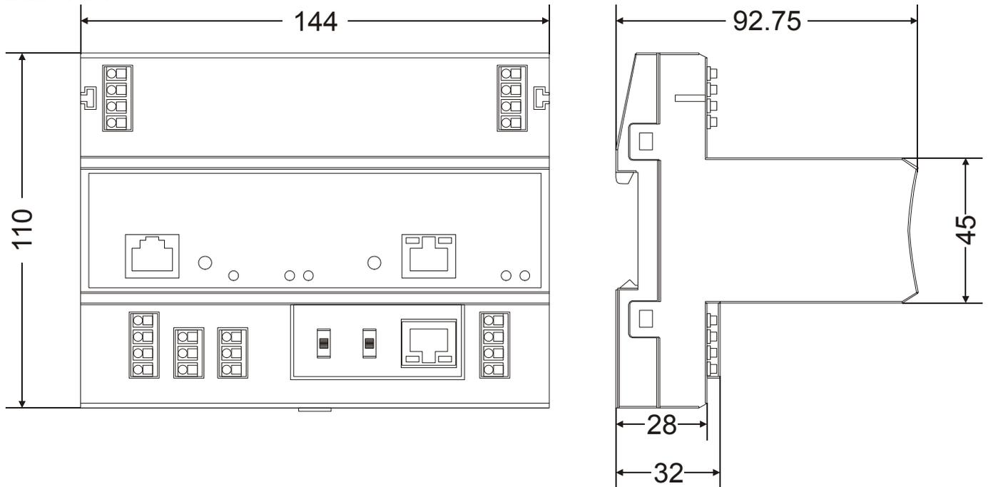
**Fig. 23. CLLIONLC01 Controller Module, outside dimensions (in mm)**
