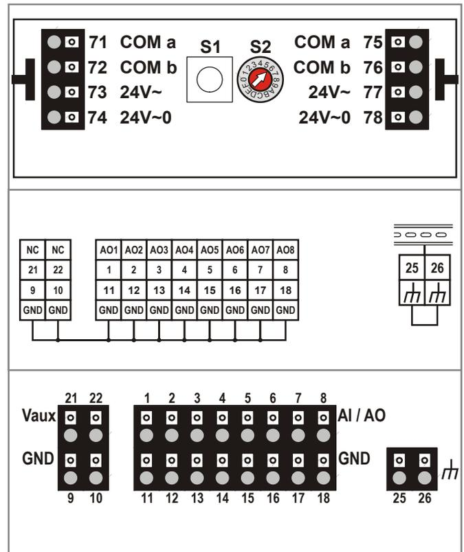
Fig. 13. LION Analog Output Modules (schematic)
