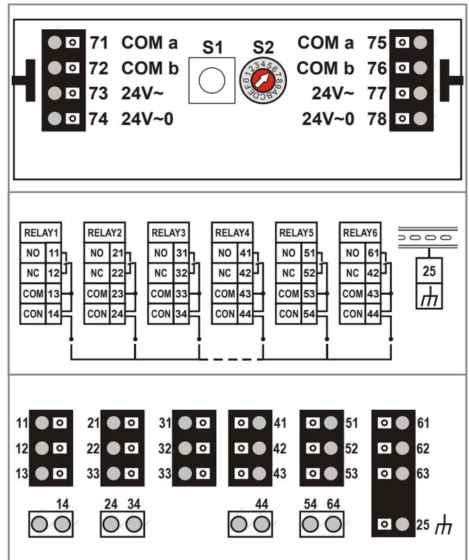
Fig. 18. LION Relay Output Modules (schematic)
