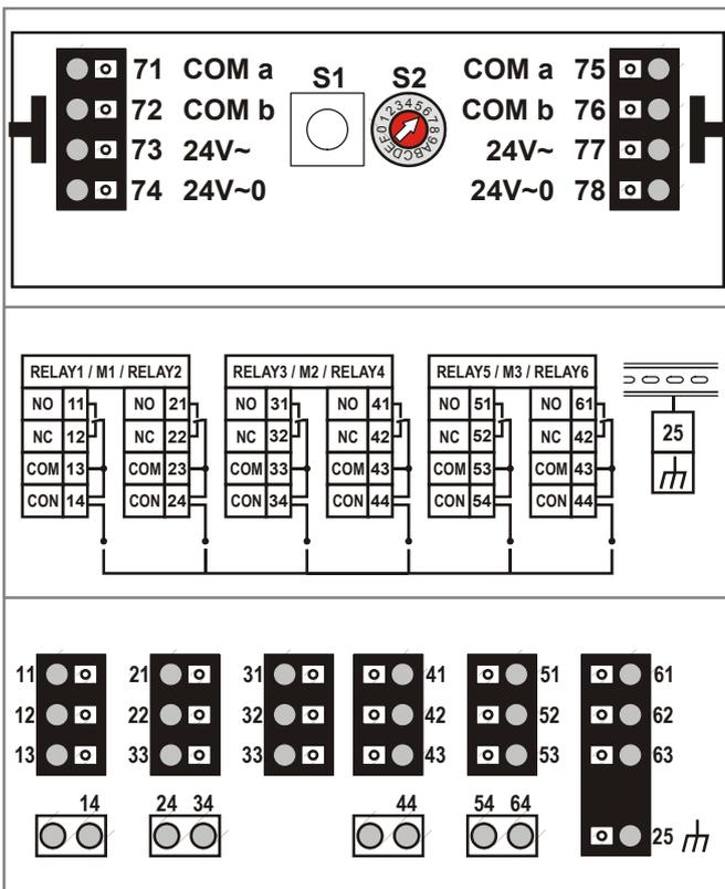
**Fig. 20. CLIOPR825A Panel Bus Floating Output Module (schematic)**
